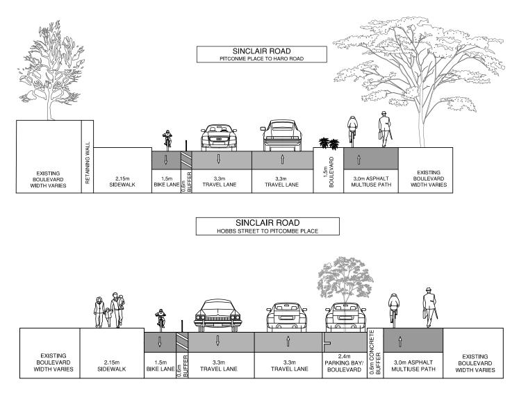
Figure 6.3: Sinclair Road Design Concept- Middle Section (Segment 2)
